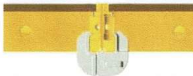
► Tying connecting panel profiles with fixed clamp
