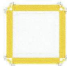
► Maximum column of 30" x 30", using universal panels with outside corners tied with fixed clamps
